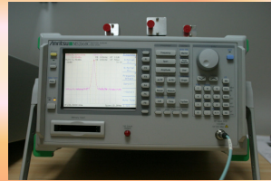
Spectrum analyzer measuring a 30 GHz signal
